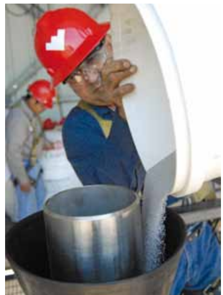
Screen is being filled and packed in Johnson Screens' packing tower.
