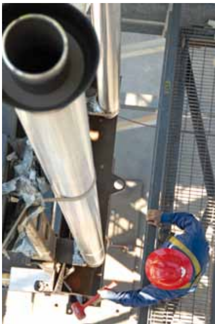
Johnson Screens' screen-packing tower is equipped with a high-intensity shaker to ensure filter media is tightly packed for optimal sand control.
