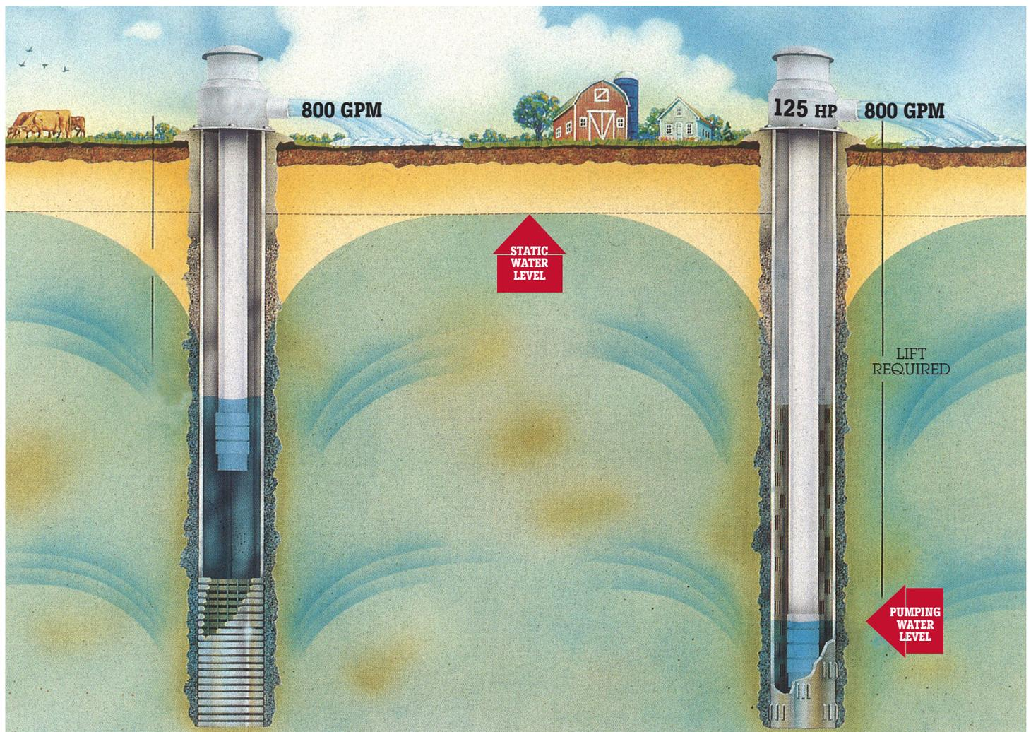
The amount of lift required on wells using Agri-screen is substantially less than wells using slotted pipe, louvered or bridge-slot screen. As a result, properly designed wells using Agri-screen requires smaller pumping units and less energy to operate. Direct savings on pump and energy costs on an individual well can range from \$1000 to \$10,000 every season.
