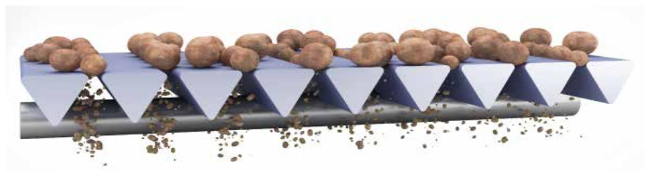
Vee-Wire® filter media retaining surface
