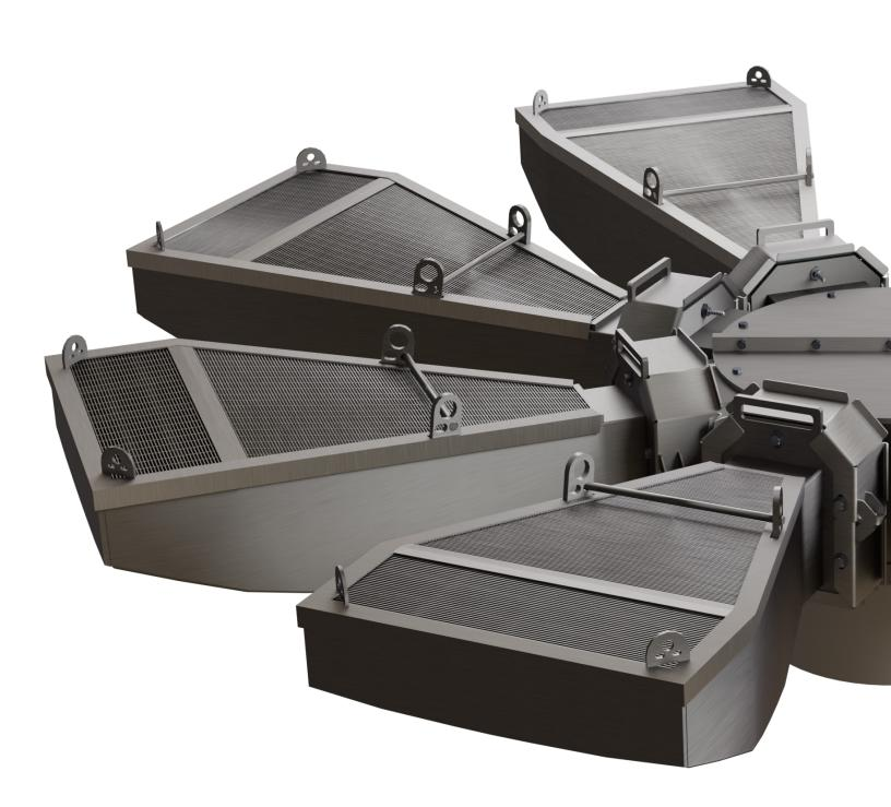
Johnson Screens' Shaped Support Grid is installed into the bottom head of hydroprocessing or gas dehydration vessels. This allows for increased media volume, increased run time, improved gas and liquid flow distribution, bed utilization and an overall more efficient process.
