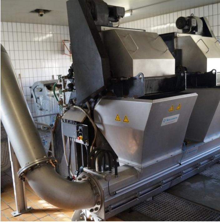
The Noggerath® screenings wash press offers a simple and reliable solution for washing, dewatering and compacting screenings from any screen. The versatility and flexible manner of the NW makes it ideal to be retrofitted into existing plants.
