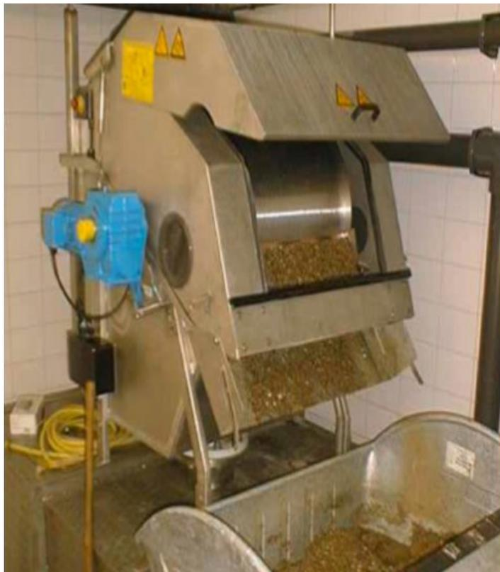
The Noggerath® Rotary Drum Screen (RSH-E) is a continuously operating screening system, with an automatic cleaning device, which separates floating, greasy and sticky solids. The RSH-E is driven by a side-mounted geared motor and an internal water spraying system is integrated into the screening drum (motor shaft designed as a hollow shaft).
