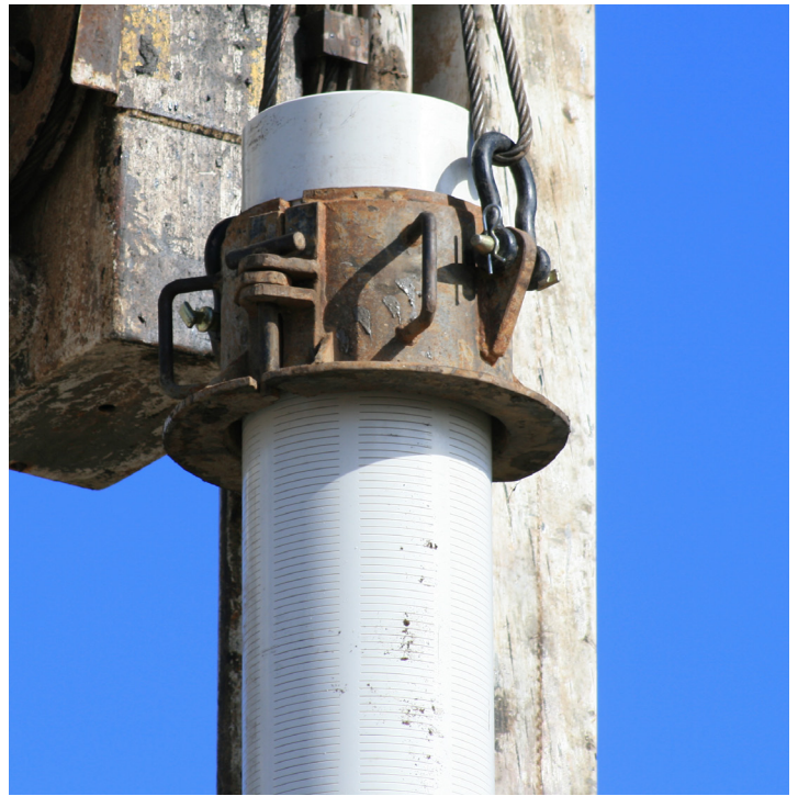
Shur-Grip machined groove allows for a quick and secure elevator connection
