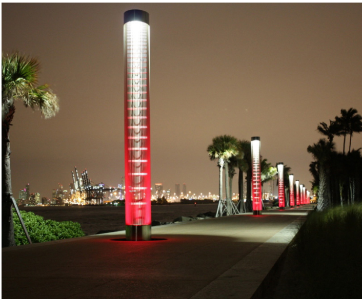
The 18 light masts that line South Pointe Park have metal halide lighting at the top of the masts, and LED lighting at the bottom. Designed with nature in mind, the ladder that runs through the middle of each light mast, shields the white metal halide light from shining out to the sea and affecting sea turtle migration.
